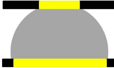
Figure 6.2 Illustration of a solder joint with large bottom bonding pad and small top bonding pad
