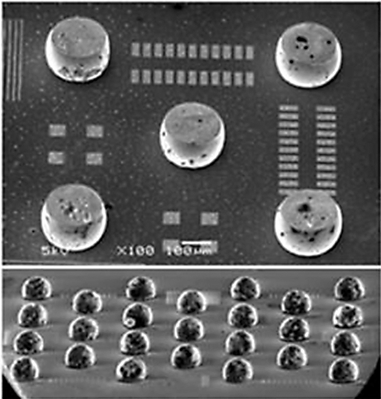
Figure 2.8 SEM images of solder bumps being plated on solder pads before (bottom) and after assembly (top)
