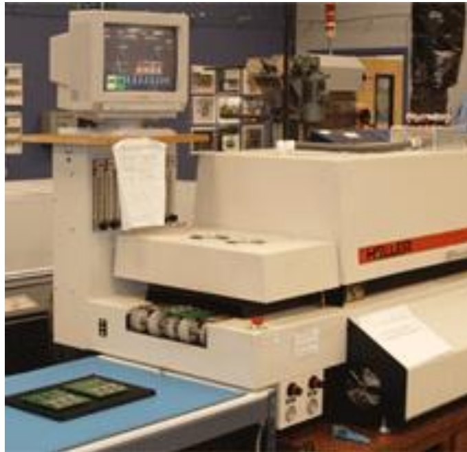
Figure 5.12 A four zone reflow oven used to test dynamic environments of an SMT manufacturing line
